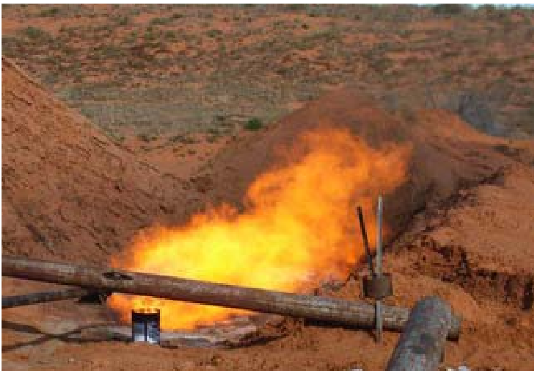
Vanessa-1 Gas Discovery – Flaring at 4.9 MMCFD at 750 PSI on ½” choke
