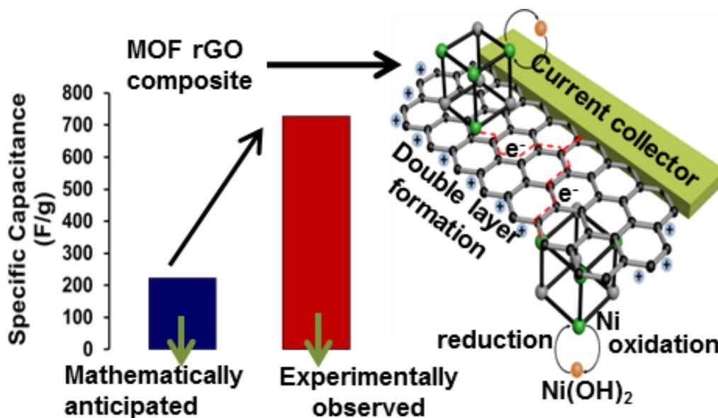
**Fig 1.** A novel electrochemical reaction and an electrochemical synergy between the MOF and reduced graphene oxide lead to a charge storage capability three times higher than the mathematically anticipated value
